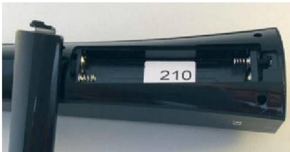
*Figure 2. Device battery holder. This accommodates up to 4 blue special 3.6 V AAA batteries. Make sure you have plenty of fully spare charged batteries at your disposal to ensure continuity of treatment.*
