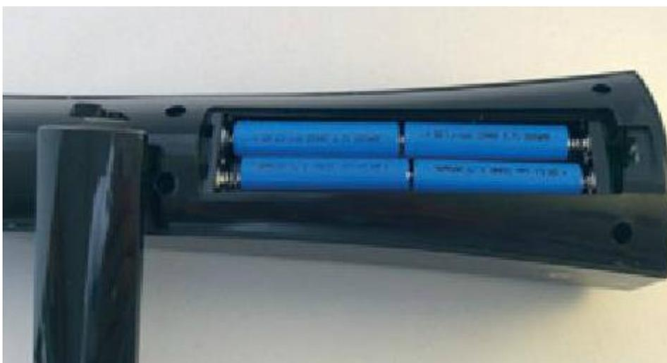
*Figure 4. Four battery configuration. The white dummy battery is not needed for this configuration. Respect polarity.*
