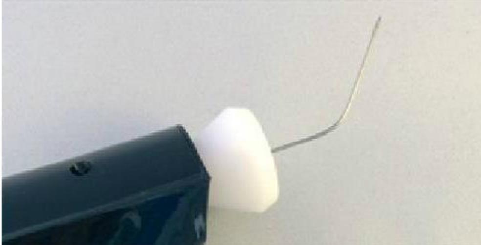
*Figure 9. The needle can be bent in order to allow ease of operation.*
