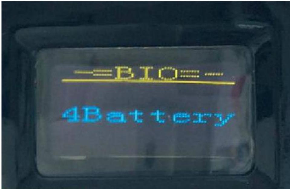
*Figure 5. Default configuration. No matter whether you place 3 or 4 batteries this is what the screen will display as soon as the batteries are placed inside the device.*
