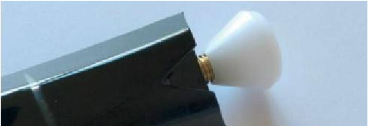
*Figure 8. The white head of the device has to be unscrewed in order to allow the needle holder to release and accommodate the needle.*
