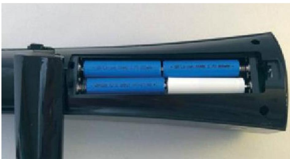
*Figure 3. Three battery configuration. The white dummy battery can be placed anywhere in the battery holder. Respect polarity.*
