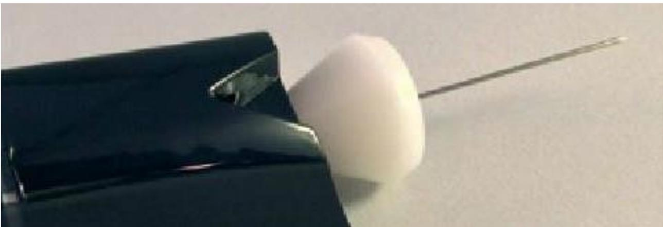
*Figure 9. Once you placed the needle inside the needle holder simply screw the white head to secure the needle. Avoid over tightening.*
