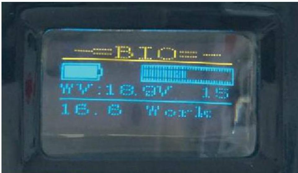
*Figure 10. Once you press the On/Off button the second time you will power up the tip of the device and you will read "Work" on the bottom right of the screen.*
