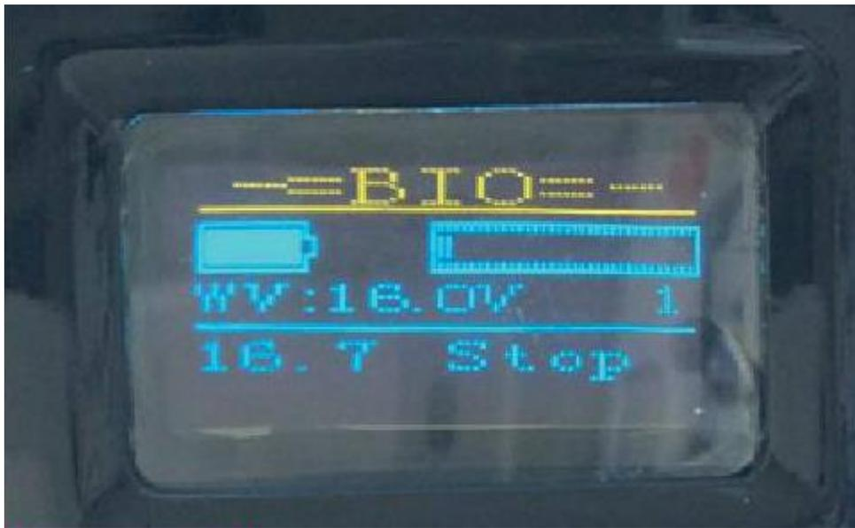
*Figure 7. This is how the screen will appear by default as soon as the device is started up by pressing the On/Off button.*
